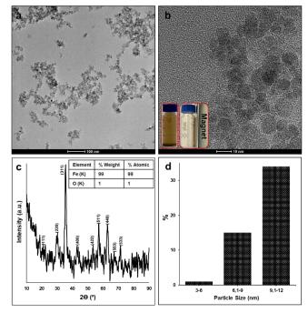
Figure 2. a-b) TEM images at different magnifications, c) XRD pattern, d) size distribution of  $Fe_3O_4$  nanoparticles.
