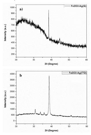
Figure 1. XRD graphs of films a) F1 and b) F2
