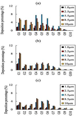
Figure 4 Deposition rates of particles of different sizes in each region of three distinct airway models: (a) Airway 1, (b) Airway 2, (c) Airway 3 (Kadota et al., 2022)
