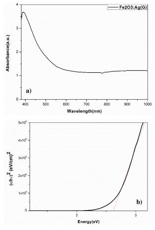
Figure 2. a) Absorbance graph of F1 and b) Bandgap graph of F1
